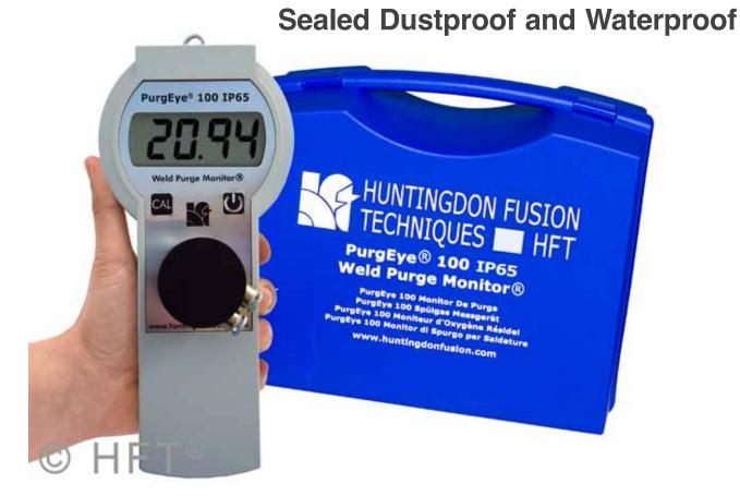
HFT<sup>®</sup> bring to the market place a World "first", and fully accredited IP65 standard rated Weld Purge Monitor<sup>®</sup>. The **PurgEye<sup>®</sup> 100** now has a dustproof and waterproof outer case that prevents the ingress of dust or moisture even to the extent of having hard water spray directed against it.
