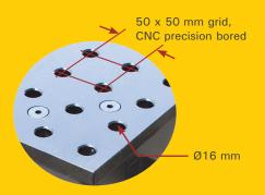
Accurately position parts in CNC precision bored 16 mm dia. holes in 50 x 50 mm spacing pattern. Rhino Package Part No.: Package Includes: Tabletop Size: Tabletop Thickness: Hole Diameter: Grid Pattern: Table Height: Static Loading Capacity: Package Gross Weight: Tabletop Life: TDQ612075-K1 Rhino Cart + 66 pc. Fixture Kit 1,200 x 750 mm 16 mm 16 mm 50 x 50 mm 910 mm 680 kg 235 kg Nitrided and black oxide table plate is **REVERSIBLE**. Weld spatter, rust and scratch resistant.
