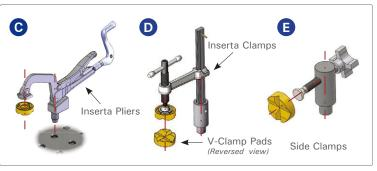
Quick hold-down clamping of flat, square, angled or round parts.
