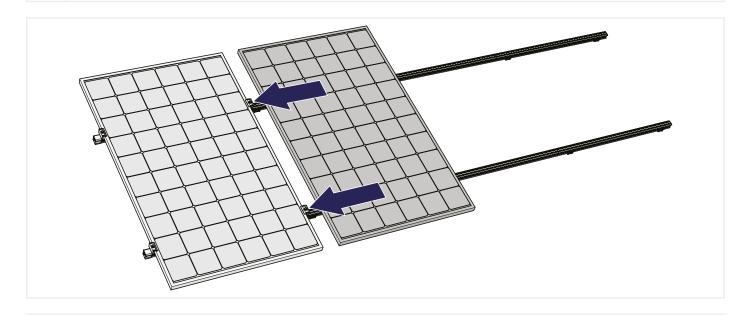
8 FASTEN THE SCREW OF THE MID CLAMPS TO SECURE THE PANEL. APPLY A TORQUE OF 16.5 NM.
