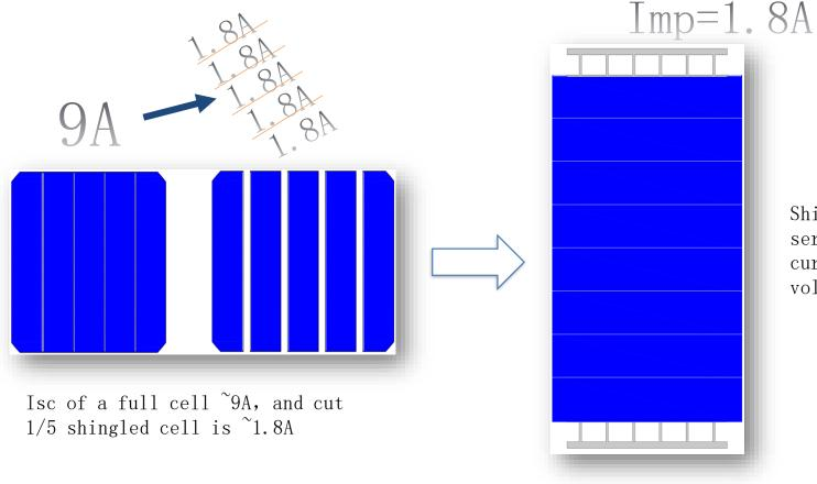
Shingles connected in series with the same current and accumulated voltages
