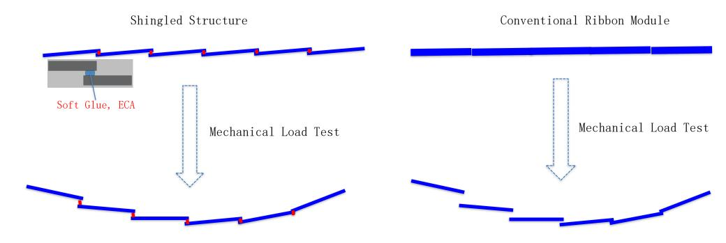
Mechanical load test: with shingled flexible cell joints and absence of metal ribbon, the shingle cell string handles load well---the flexible adhesive acts as a shock buffer and absorbs bending energy. In comparison the ribbon soldering joints of conventional cell strings develop cell cracks easily under external load.
