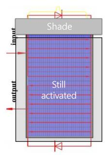
• Hyundai shingled modules are made in **parallel** circuits and brickwork layout design which will make less influences from shade compared with full cell & half-cut cell modules.
