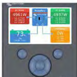
Color Control GX, showing a PV application
