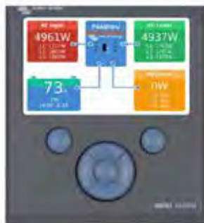
Color Control GX, showing a PV application
