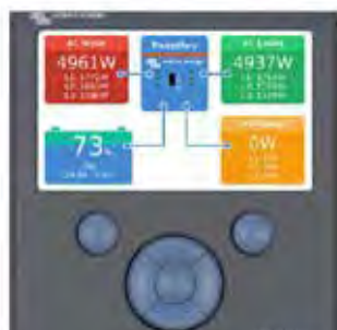
Color Control GX, showing a PV application
