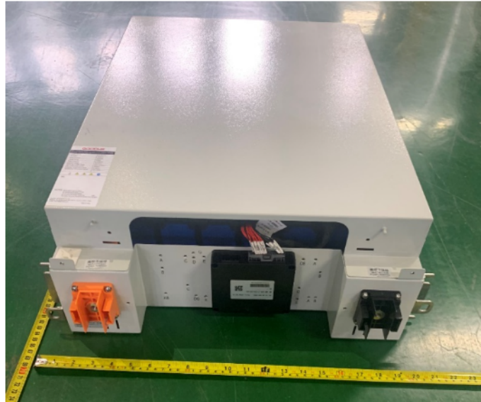
图 1. 可充电锂电池包 LX C9.2-10 Fig.1 Picture of Rechargeable Li-ion Battery Module LX C9.2-10
