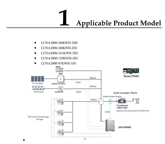
Huawei C&I Smart String Energy Storage (ESSs for short) Products LUNA2000B series are applicable to industrial and commercial scenarios. They work with the SmartPCS, DCDC and SACU. The SmartPCS is connected to the pack controller DCDC, and charges batteries when the power grid is sufficient. When the power grid needs to be output, the SmartPCS outputs the stored battery energy to loads for use.
