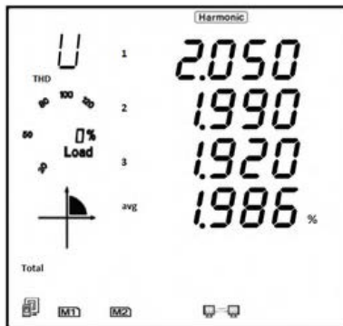
Figure 3-25 Harmonic Distortion Reading
