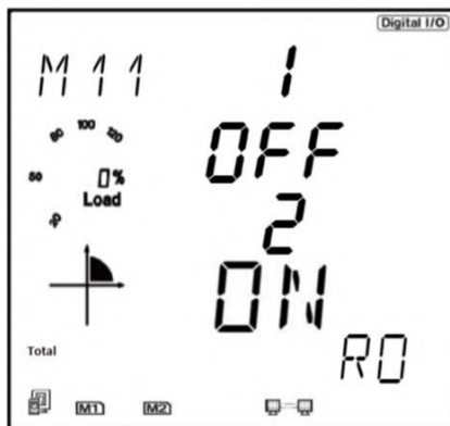
Figure 5-26 Relay Output Status Readings
