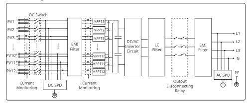
The circuit diagram of GW73KLV-HT/GW110K-HT/GW120K-HT is as follows.
