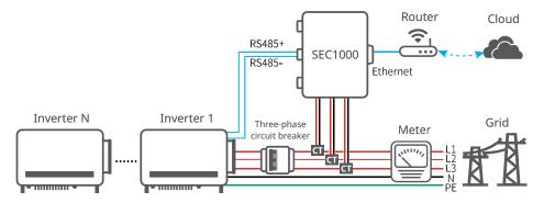
After completing cable connections, set related parameters via LCD or SolarGo app to enable export power limit control or output power limit control.
