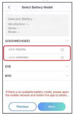
Click "GOODWE(HIGEE)" and then select the proper battery model matching with the communication method on "Select Battery Model" page of the PV Master App.
