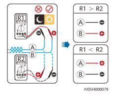
2. Connect the PV string cables to the inverter.
