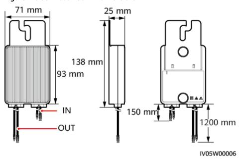
**Figure 2-4** SUN2000-450W-P2/SUN2000-600W-P (short input power cable) dimensions
