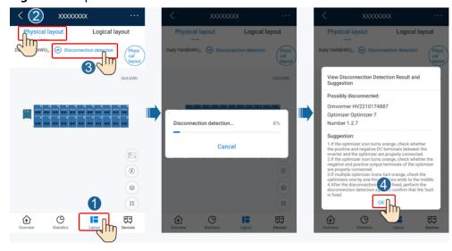
Figure 5-1 Optimizer disconnection detection
