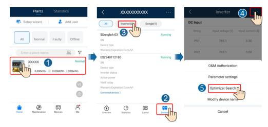
**Step 7** Choose **Devices > Connected devices > Optimizer**, tap **Optimizer No.**, select the faulty optimizer, tap **Device Replacement**, and replace the optimizer as prompted.
