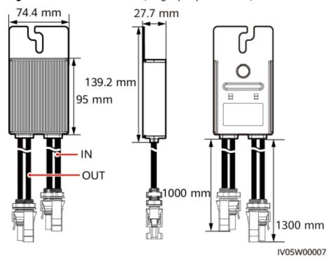
Figure 2-5 SUN2000-600W-P (long input power cable) dimensions
