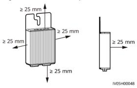
Figure 4-1 Clearance requirements
