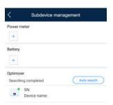
**Step 7** On the device commissioning screen, choose **Maintenance** > **Optimizer layout**, select the corresponding PV module, and bind the new optimizer according to the recorded mapping information. Tap **Submit**.
