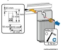
• Method 2: Install the optimizer to the PV module frame using a bolt assembly.
