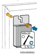
Method 3: Install the optimizer to the PV module frame using a frame mounting bracket (front installation).
