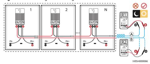
Figure 6-1 Measuring the PV string resistance
