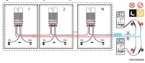
Figure 4-7 Measuring the PV string resistance
