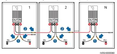
**Step 2** Use a multimeter to measure the resistance of the PV string when the irradiance is adequate. The resistance level of the multimeter affects the measurement precision of the PV string output resistance. Select the minimum resistance level that meets the measurement requirements.
