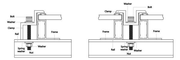
Figure 7. Specific installation of clamps
