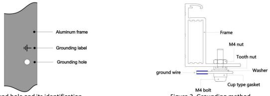
Figure 1. Ground hole and its identification
