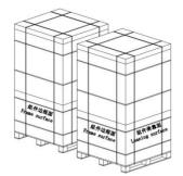
Unpacking the reclining surface needs to be close to a solid wall or another pallet of intact components of the same size
