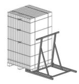
Place a support bracket on either of the recline surfaces of the assembly and remove the three transverse steel strips from the upper part of the assembly with a cutter
