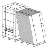
Gently push the module so that it leans against the support, removing the vertical strip of plastic steel
