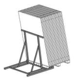
Remove all modules in sequence to complete module unpacking
