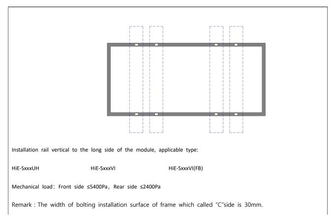
Inner four mounting hole installation (mounting hole size: 9\*14mm)
