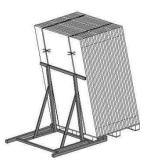
Gently push the assembly so that it leans against the support frame and remove the vertical steel strip
