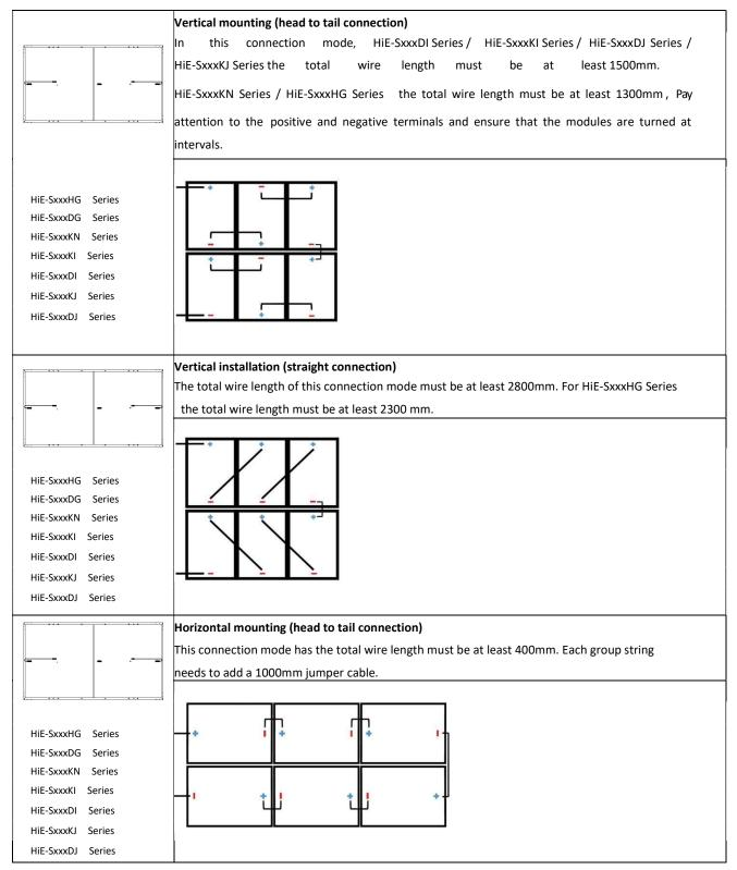
Note: 1. Total wire length means positive plus negative cables length.
