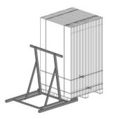
Two people stand on the frame surface of the module to hold the component, while the other person cuts the lower two transverse plastic steel packing belts
