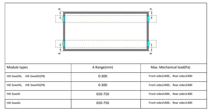
Six Clamps mounting on long side of frame and rails perpendicularly to the long side frame, the middle rail is located in the center of the module
