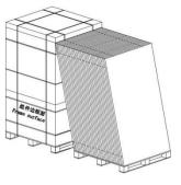
Remove all modules in sequence to complete module unpacking
