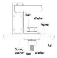
Figure 6. Bolt installation methods
