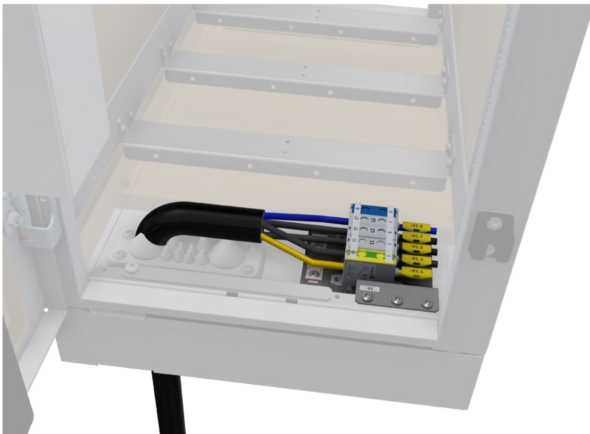
Figure 4.5 AC mains cable - TN-S (230/400Vac) network
