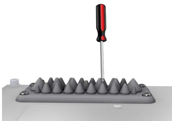
Figure 4.2 Cable glands preparation
