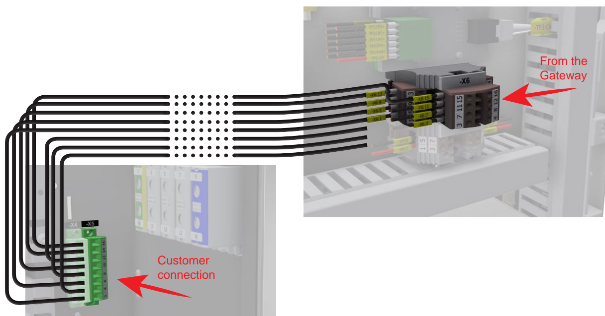
Figure 4.22 Customer spare terminals connection
