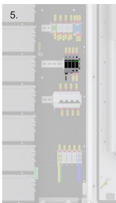
Figure 4.7 Disconnecting wires from SPD -FA1
