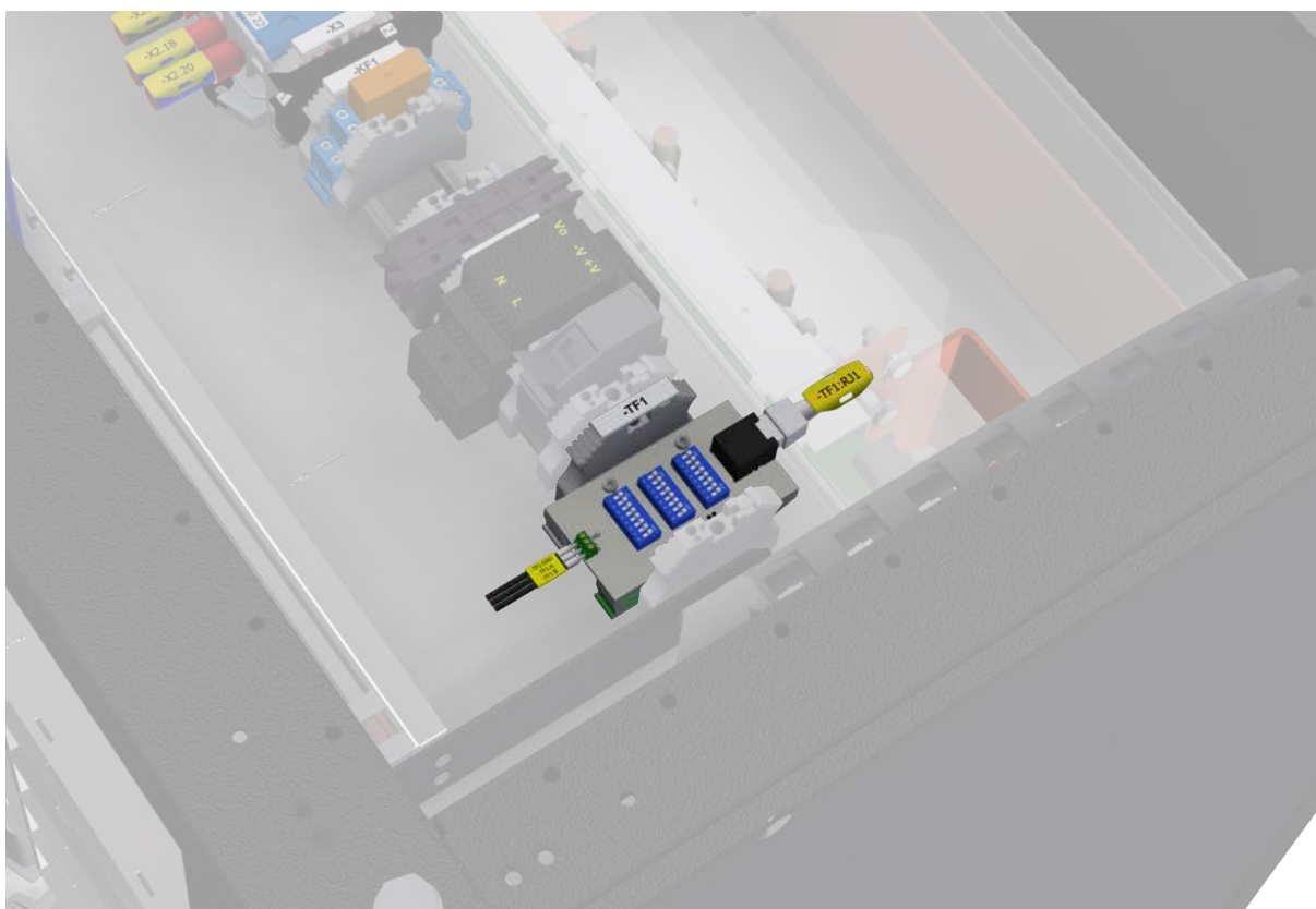
Figure 4.24 Battery Com converter (-TF1)
