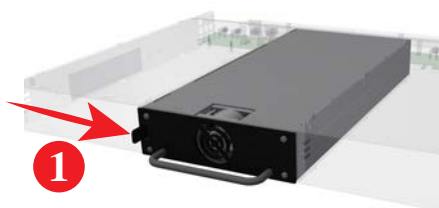
Figure 4.27 Unlock the ratchet
