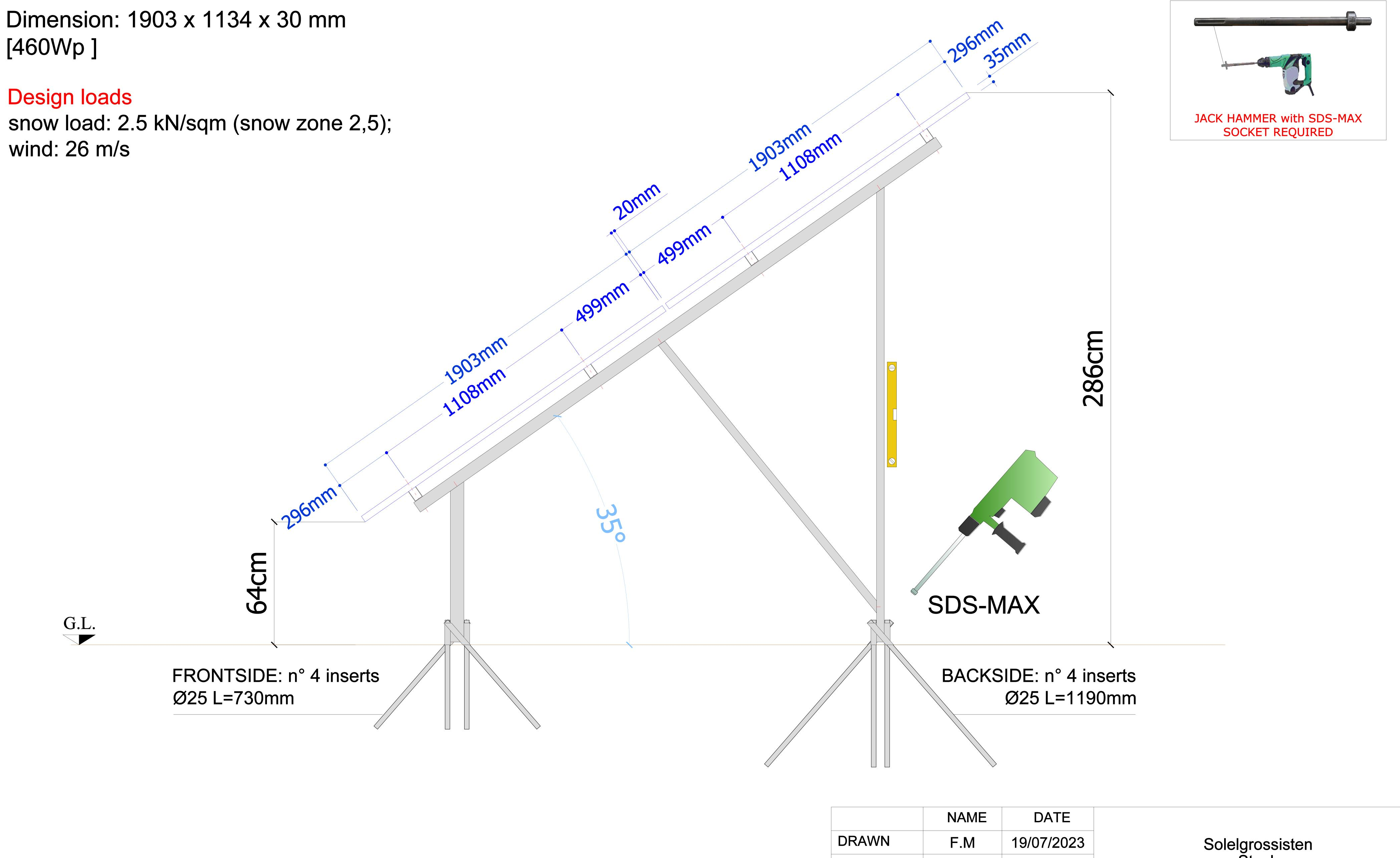
Driving-in the inserts to the ground through guides placed at the base of the frames, using a jack-hammer with SDS-MAX tool tip or a common hammer, only when all the structure is installed and it has checked that the spirit level giving the transverse orientation of the structure indicates the horizontal.
