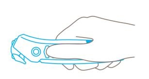
For the best possible grip, place your thumb on the **three ribs**. The soft-grip further limits the possibility of slipping.
