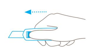
Use the slider to **engage the blade** for cutting.
