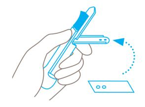
Use your index finger to slowly **fold out the blade holder downwards**. Use the other hand to remove the blade to either replace it or turn it around (for left handers).
