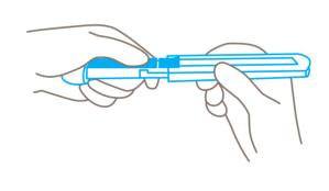
When the slider and blade leave the handle, position your index finger under the blue blade holder to hold it tight.
