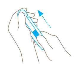
Use the slider to **push** the plastic insert back and out of the handle. **Don't** pull the insert while holding onto the slider.
