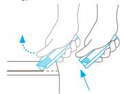
**Automatic blade retraction – a high degree of safety**The automatic blade retraction of the SECUNORM
