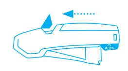
Pull the **blade change button** to the top and release the lever. Blade and blade holder will come out of the handle.
