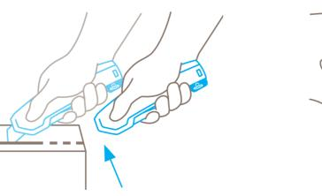
The blade immediately retracts into the handle the moment cutting ceases. Even when the lever is **still being squeezed**.
