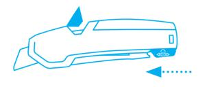
Secure the lever with the safety device and turn the handle so that the **transparent blade cover is facing upwards**.
