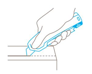
Unlock the lever by **pulling** the safety device. Squeeze the lever to extend the blade. Now you can cut.
