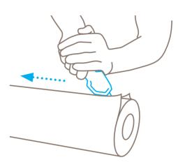
For **power cutting**, push the lever and cut while pulling. Use second hand for reinforcement.
