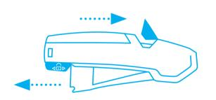
Slide the lock to the rear position, so that the **lever can be released** again. **Then** push the blade change button back into the handle and continue cutting.
