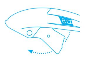
**Swing the lever out** of the handle and flip open the blade cover.
