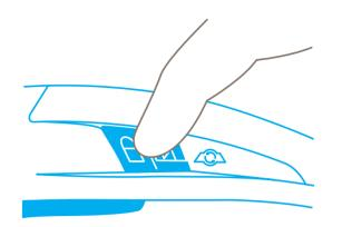
To prevent unintentional blade activation, always lock the safety knife by pressing downwards on the lock symbol.
