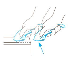
The blade immediately retracts into the handle the moment cutting ceases. Even when the lever is **still being squeezed**.
