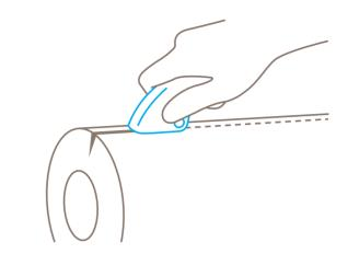
Use the underside of the knife head as a supporting surface to work ergonomically and efficiently.
