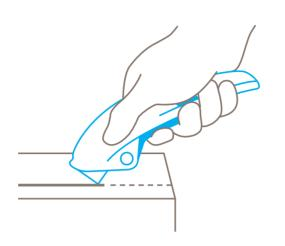
To engage the blade, unlock the safety knife and squeeze the lever. Now you can cut.
