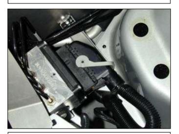
e. Plug in the ABS wiring harness back into the ABS control module.
