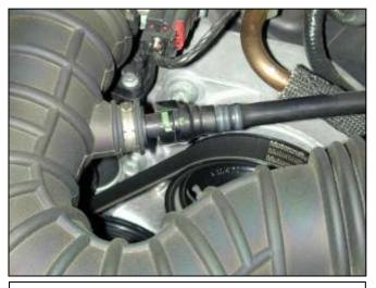
c. Loosen the hose clamp on the throttle body attached to the stock intake hose. Unplug the plastic breather hose connected to the intake hose. This is done by sliding the green retaining clip until the hose is free from the nipple.
