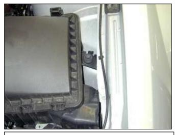
d. Remove the bolt securing the stock air box to the vehicle. Lift up on the stock air box until it is free from the vehicle.
