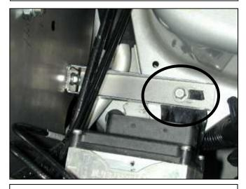
d. Install the lower heat shield mount by using the previously removed lower ABS mount bolt. Use the supplied M6 bolt, nut, and washer to secure the lower mount to the heat shield.
