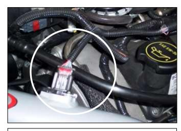
r. Plug in the wire harness into the MAF sensor.
