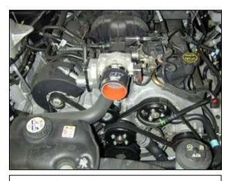
g. Install the supplied adapter hose onto the throttle body as shown using the #48 hose clamp.
