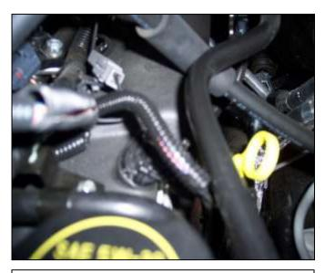
o. Place supplied convoluted slit covering over the remaining two wires as indicated in the picture above.
