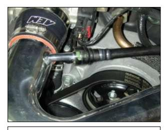
j. Attach the stock plastic breather hose by pushing it over the aluminum nipple on the AEM<sup>®</sup> intake pipe until it snaps into place.
