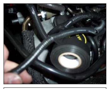
p. Wrap the factory convoluted slit covering with electrical tape to secure the wiring from potential damage.
