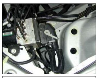
f. If your vehicle is not equipped with ABS, proceed to Step 3. Remove the ABS wire harness from the ABS control unit. This is done by pushing in on the locking button and rotating the latch mechanism toward the engine.
