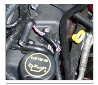
I. Remove the wires from the convoluted slit and cut the electrical tape to locate MAF sensor wires.
