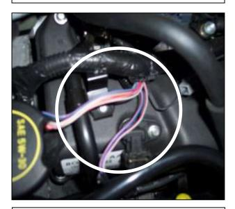
m. Pull MAF sensor plug towards MAF sensor.
