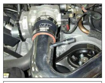
h. Insert the inlet pipe into the coupler installed on the throttle body as shown.
