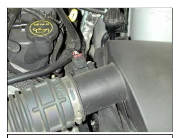
b. Unplug the wire harness from the mass air flow (MAF) sensor.
