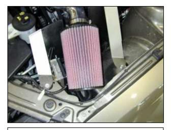
k. Install the AEM<sup>®</sup> air filter onto the end of the intake pipe. Push the air filter over the intake pipe until the stop in the air filter is reached. Secure the air filter onto the intake pipe with the supplied hose clamp.
