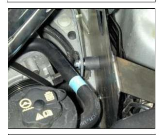
i. Align the mounting bracket with the rubber mount on the heat shield. Install the M8 washer and serrated nut onto the rubber mount. Leave slightly loose for adjustment.
