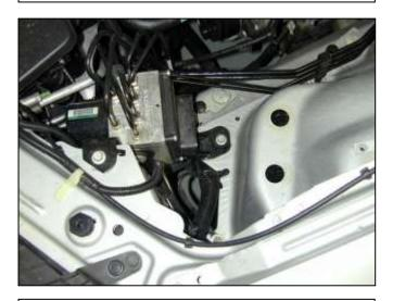
g. Move the harness out of the way and remove the upper and lower bolts securing the ABS unit to the chassis as shown. Set these bolts aside for now, they will be used during the AEM<sup>®</sup> intake system installation.
