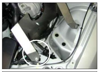
c. Install the heat shield into the engine compartment by carefully sliding it under the AC lines and aligning the two mounting arms with the holes in the fender and upper ABS mount. Secure using the previously removed bolt for the ABS housing and supplied M6 bolt and washer.
