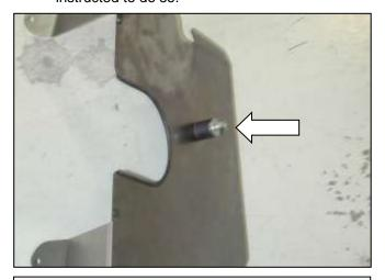
b. Install the supplied rubber mount onto the AEM® heat shield using one of the supplied washers and locknuts. Install the rubber edge trim around the pipe opening as shown.
