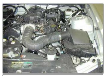
Factory air box system installed
