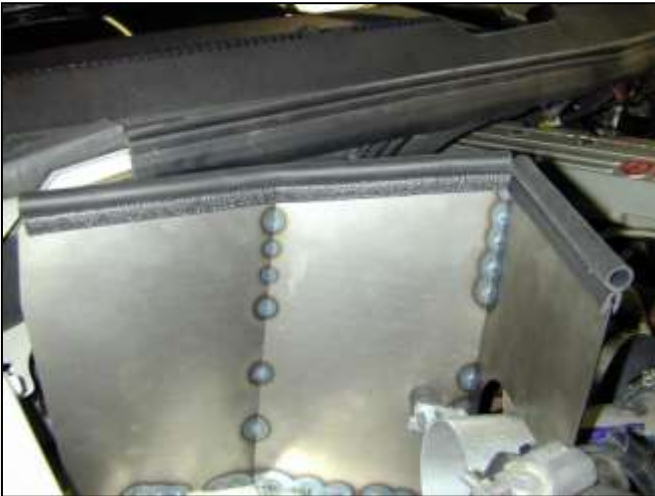
h. Install rubber gaskets to top of heat shield.
