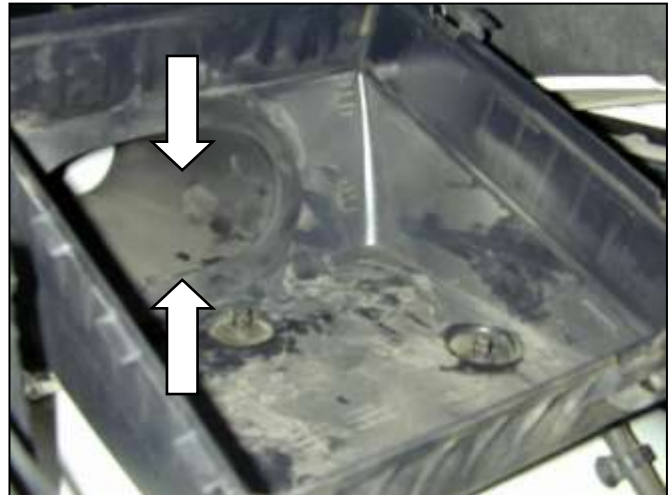
d. Remove snorkel by squeezing middle together while pulling towards center of the vehicle.
