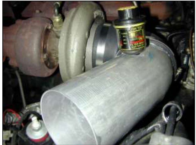
i. Confirm that the inlet pipe is free of obstructions. Attach inlet pipe onto elbow.
