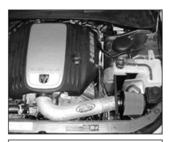
AEM® intake system installed
