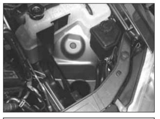
c. Insert the heat shield. You will need to check all mounting surfaces in the following steps.
