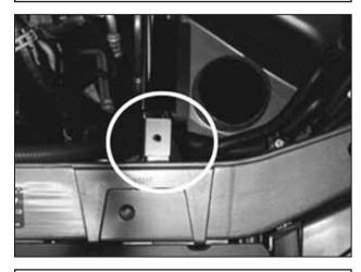
f. Check the final tab alignment. Insert the factory bolt removed in step 2g to secure this tab.
