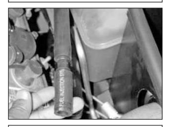
s. Insert the other end of the plastic connector into the factory crank case breather hose.
