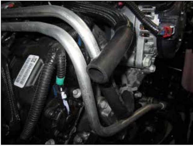
c. Disconnect the rubber breather hose from the stock air box lid.
