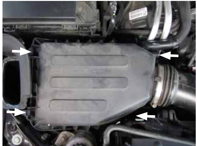
b. Release the 4 clamps on the stock airbox lid.
