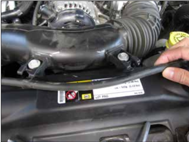
e. Release the coolant bypass hose from the finger clamps on the stock intake tube.
