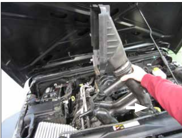
g. Pull up on the stock intake tube and lid assembly until the IAT sensor is visible and accessible.
