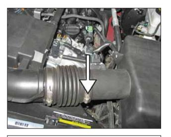
b. Loosen the hose clamp on the air box side.
