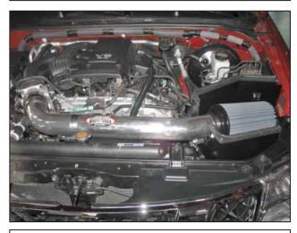
AEM® intake system installed
