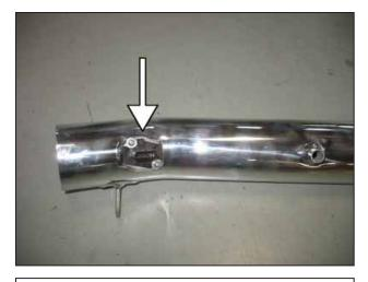
f. Insert the MAF sensor and secure with the factory hardware as shown.
