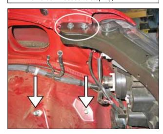
j. Remove the air box mounting bolts Also remove the two bolts from the radiator support.
