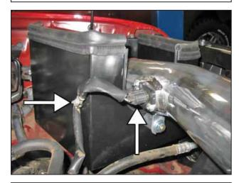
j. Plug in the MAF sensor harness into the MAF sensor. Secure the MAF sensor wire harness to the heat shield as shown.
