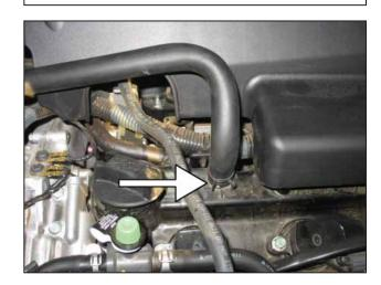
d. Remove the crank case breather tube from the valve cover; save the sping clamp for later use.
