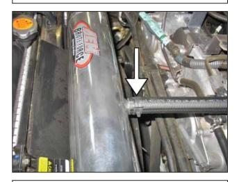
k. Attach the crank case breather hose to the intake pipe and secure with the factory spring clamp.
