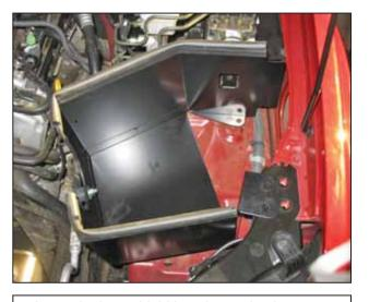
c. Insert the heat shield into the engine bay.
