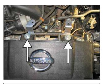
f. Remove the remaining bolts securing the air inlet tube, then remove the air inlet tube from the vehicle.
