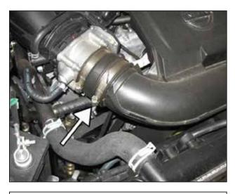
a. Loosen the hose clamp at the inlet tube side only.
