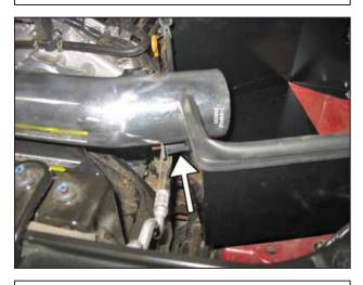
h. Line up the intake pipe's bracket with the rubber mount installed on the heat shield. Ensure the intake pipe has proper clearance, then secure the hose clamp at the throttle body.
