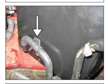
o. Secure the transmission breather hose to the heat shield with the zip tie and mount as shown.
