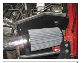
m. Attach the air filter and secure to the intake pipe. Check for clearance around the air filter.
