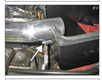
i. Secure the bracket to the rubber mount with the provided washer and nut.
