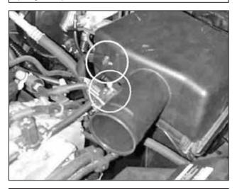
g. Unplug the MAF sensor and remove the MAF sensor harness.
