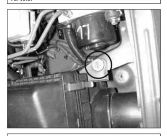
h. Remove the rear mounting bolt to the air box. Remove the air box from the engine bay.
