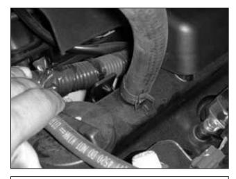
I. Attach and secure the other end of the breather hose to the crank case vent, secure with the factory hose clamp.
