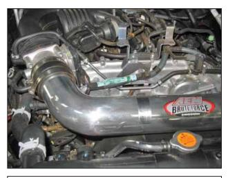
g. Insert the intake pipe into the coupler, secure in place, but do not completely tighten the hose clamps.
