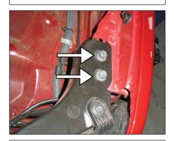
e. Secure the tab at the radiator support with the stock bolts as shown.
