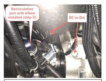
(d. cont.) bolt. Ensure that the O-ring remains seated. Torque both bolts to 80 in-lbs and intercooler hose clamps to 30 in-lbs.
