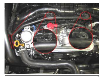
h. Remove the clips retaining the line shown above and insert the included zip ties securing them to the line as shown (offset to the right) to protect it from the heat of the charge pipe.
