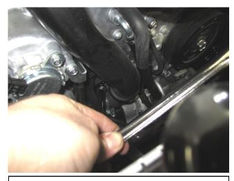
c. Use the 12mm socket with a U-joint and extension to remove the bolts securing the charge pipe flange to the turbocharger.
