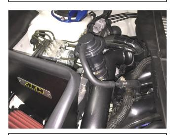
g. Using hose removed in step 2d and connector (Item 10), install your valve and assemble the vacuum supply line as shown.
