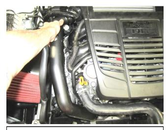
d. Lower your new AEM charge pipe into position and install beginning with the top end at the intercooler and slide lower end into position to install the other flange
