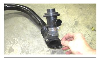
b. Remove the O-ring from the factory charge pipe and install into your new AEM charge pipe with care to orient the tab in its corresponding groove.
