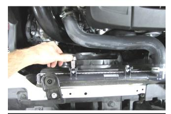
b. Remove fan using a 10mm socket as shown. Once the two top bolts are removed and the power harness at the bottom is disconnected, the fan can be lifted out of the engine compartment and set aside.
