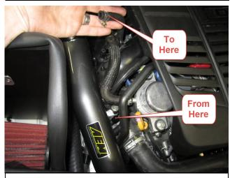
f. Re-route vacuum line through the intake manifold as shown above. Use the other included cap to protect the exposed steel line if desired.
