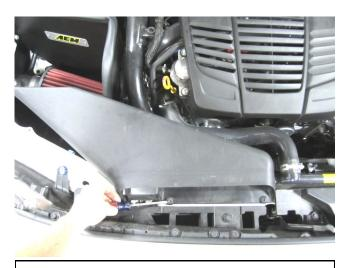
a. Remove factory fresh air inlet duct
