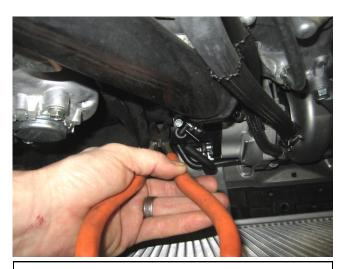
g. Using pliers, disengage the spring clamp securing the valve to the intake housing and slide it down.
