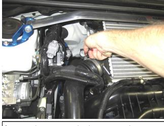
f. Loosen clamp securing the charge pipe to the intercooler enough to move the clamp off of the joint.
