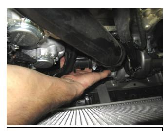
h. Lift straight up on the valve outlet while supporting the inlet to remove the factory charge pipe from the engine.
