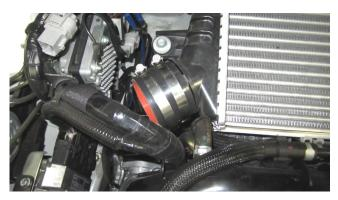
a. Install the 2.75" coupler onto the intercooler inlet with its corresponding hose clamps. Do not tighten.
