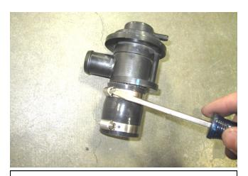
e. Loosely install the smaller coupler and clamps onto your valve of choice (factory valve shown).
