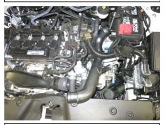
g. Insert the AEM charge pipe in the orientation shown above.
