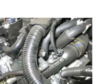
c. Disconnect the manifold absolute pressure (MAP) sensor and intake air temperature (IAT) sensor harnesses.
