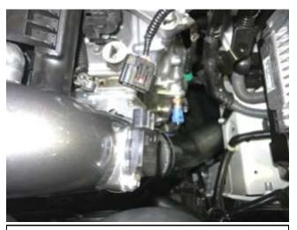
a. Disconnect mass air flow (MAF) sensor harness.
