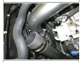
j. Insert the lower end of the pipe into the intercooler hose. It may help to spray the end of the pipe with soapy water. Alternatively, you can heat the hose end with a heat gun or blow dryer. Do not tighten the hose clamp yet.
