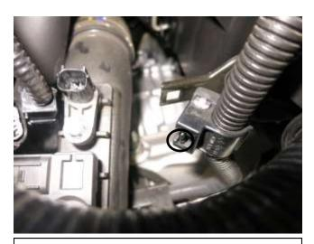
i. Pull on the small tab, circled above, then pull the harness from its mounting bracket.
