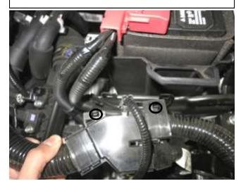
h. Pull on the (2) small tabs, circled above, then pull the engine harness from its mounting bracket.
