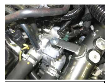
k. Adjust the charge pipe for best fitment. Once you are satisfied, fasten the mounting bracket to the rubber mount with the supplied washer and nut. Also, tighten the hose clamps at the throttle body coupler and intercooler hose to 30 in-lbs. You may also remove the tape applied in steps 3a and b at this time.
