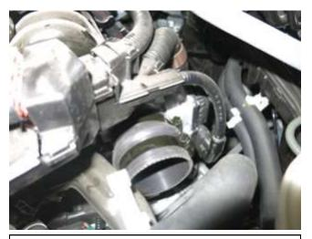
e. Install the hump hose coupler onto the throttle body, with the supplied hose clamps. Tighten the hose clamp on the throttle body side to 30 in-lbs.
