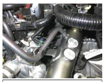
I. Install the vacuum hose to the nipple and secure with the factory spring clamp. Then, reattach the plastic clip to the mounting bracket.
