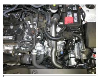
n. Begin removal of the charge pipe from the engine bay by rotating the pipe counter-clockwise. Refer to image above for the desired orientation.
