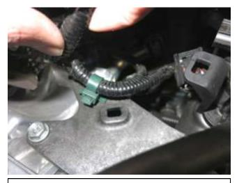
e. Use a small flat head to pry the harness mount from the stock charge pipe mounting bracket.
