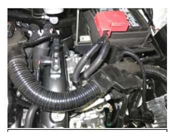
n. Reattach the (2) harnesses to the mounting bracket.
