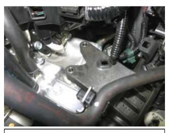
f. Use a 10mm socket to remove the (2) M6 bolts fastening the stock charge pipe to the engine block. Do not discard this hardware.
