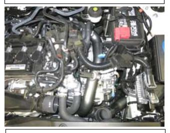
h. Rotate the pipe counter-clockwise as you push it towards the rear of the vehicle. Lower the bottom end of the pipe past the radiator shroud and radiator hose.
