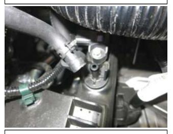
d. Use pliers to pinch the spring clamp and pull the vacuum hose from the stock charge pipe nipple.
