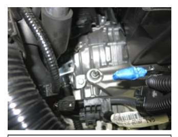
a. Before commencing the install of your AEM charge pipe, wrap the end of the bracket, shown above, in tape. This will protect the pipe from scratches as you maneuver it into place.
