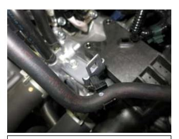
j. Pinch the tabs on the plastic clip holding the vacuum hose you disconnected in step 2d, then pull the clip from the mounting bracket. Move the hose aside.
