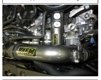
p. Reinstall the upper AEM intake tube. Make sure it does not contact the charge pipe. Finally, reconnect the MAF sensor harness.
