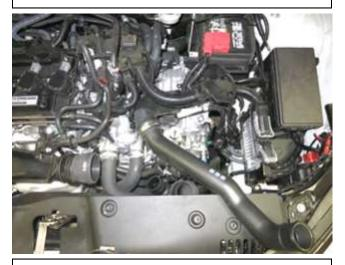
o. Lift the bottom end of the charge pipe over the radiator shroud as you continue to rotate (counter-clockwise) and pull the pipe towards the front of the vehicle. Do not discard the stock charge pipe once it's removed.
