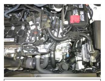
b. Loosen the hose clamps securing the upper AEM intake tube; one on the turbo inlet pipe coupler and one on the upper and lower intake tube coupler. Then, pull off the upper intake tube.
