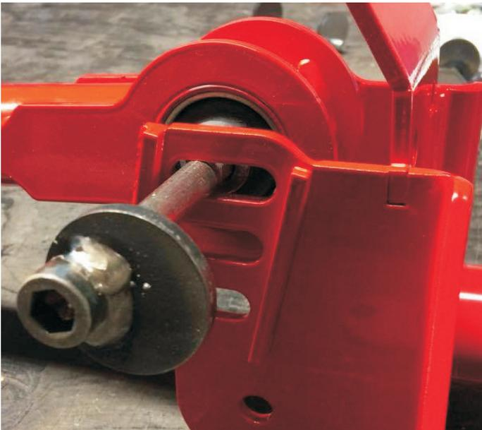
**Install the upper strut in the top slot with the specialbolt**
