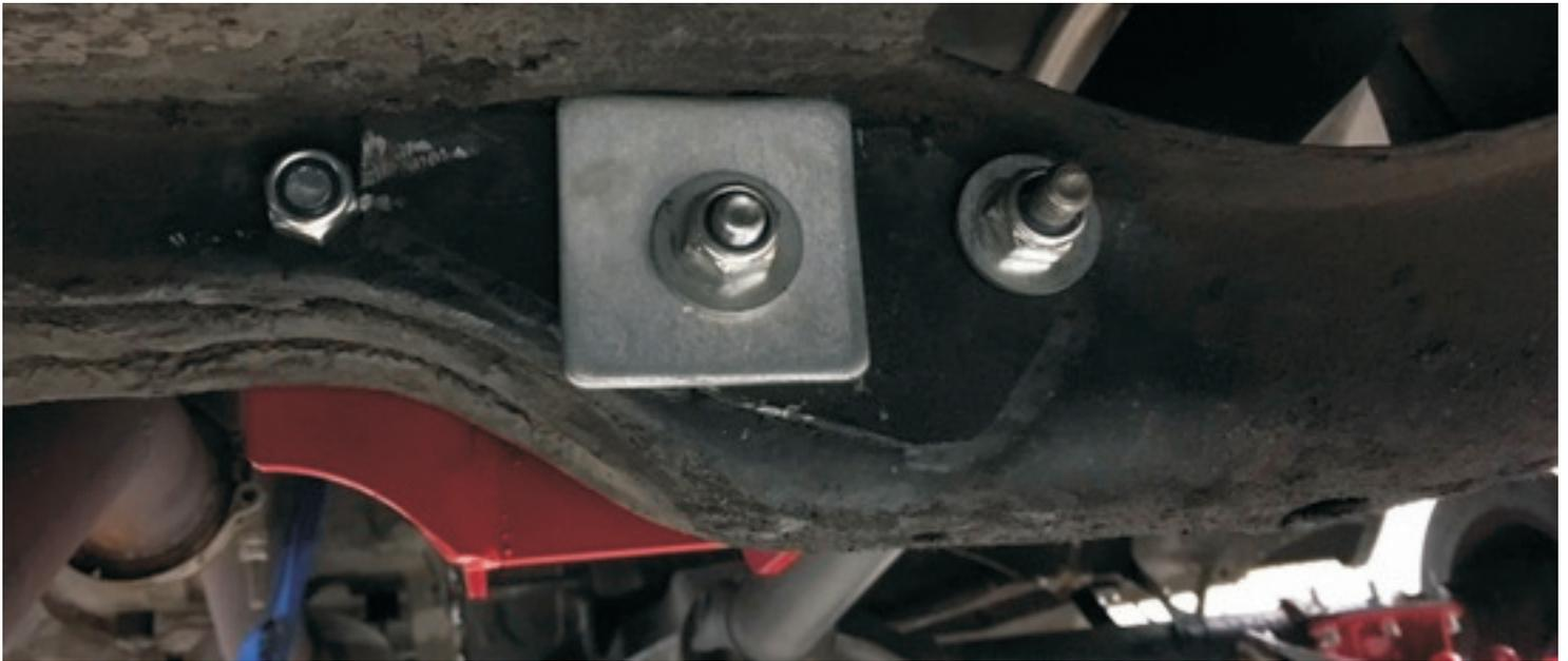
**Reinforce the back of the beam as much as you think it is needed. Use supplied reinforceplate on the inside of the car**
