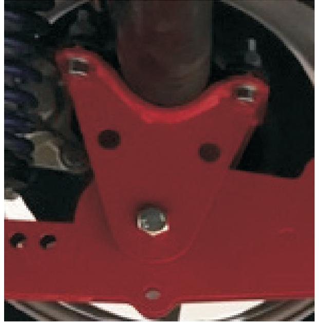
**Weld the plate on the rear axel
