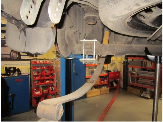
6. Using a 10mm spanner and suitable pliers undo the nut and remove the location pin from the leaf spring.
