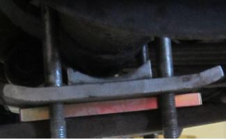
10. Now refit the oem plate and the 4 nuts. Lower the caddy to the ground. You should now have a centred rear axle.
