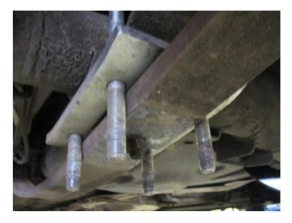
5. Using two 18mm spanners remove the bolt at the rear of the leaf spring as seen below.
