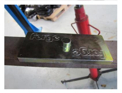
9. With the offset plate in the correct position lift the leaf spring back into place ensuring the pin locates inside the hole. Refit the bolt at the rear of the leaf spring as seen in step 4.
