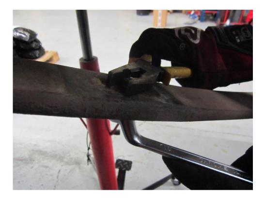
7. Insert the supplied location pin in to the hole and tap it down to the shoulder.
