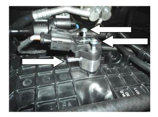
Fit the boost gauge take off using the longer screws provided. (Allen head bolts TTRS) Then connect the vacuum tubing to the take off and route to the boost gauge(not supplied)
