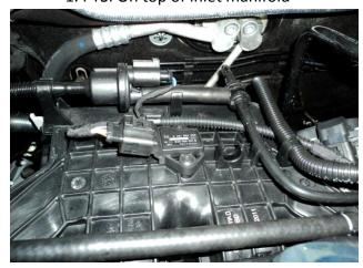
Remove the two T25 Torx head screws (Allen head bolts TTRS) and remove the map sensor
