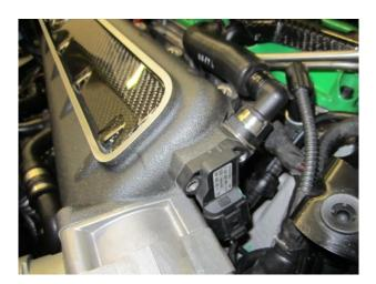
1.2 TSI On top of inlet manifold
