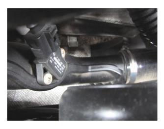
1.4 TSI On top of inlet manifold
