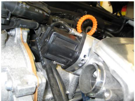
9. Once the valve is tightened down, replace the intake pipe work in the reverse sequence to above. Try the engine cover on the locating pins to make sure it clips down. If it doesn't, remove the rubber shield from around the dipstick and using a long reach 13mm socket, undo the locating pin from the block.
