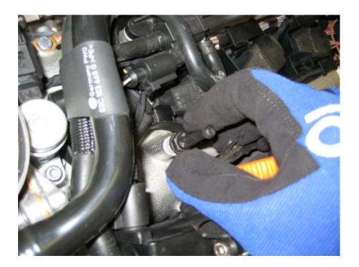
10. Using the M6 washers supplied, place them underneath the pin to raise its height until the engine cover can be clipped in. Once you are happy, replace the rubber cover for the dip stick over the pin and fit the cover for a final time.
