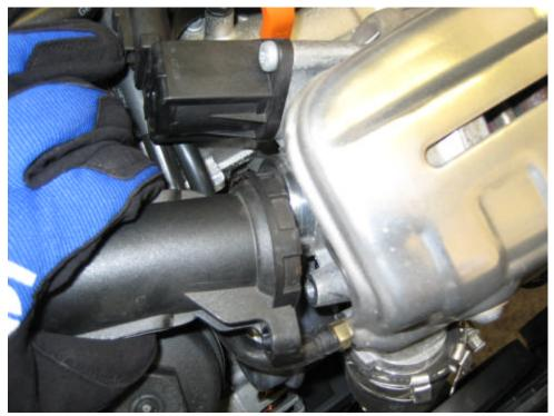
Now the turbo end of the hose is loose, it should be easy to separate the intake hose at the other end. Remove the breather hose which you loosened the clamp for in part 3, and lift the intake hose off the vehicle. You should now have enough room to work on the dump valve.
