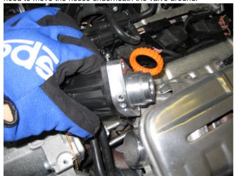
Use the two longer allen head bolts supplied to fit the valve back to the turbo. Tighten them with a 5mm allen key, and again access is limited to the bottom bolt.
