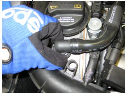
5. Remove the T30 screw holding the intake hose to the turbocharger, then the T30 screw supporting the pipe to the block, and the two T30 screws at the join between the intake pipes. Once these last two screws have been removed, you can pull off the clamp that secures the two hoses together.
