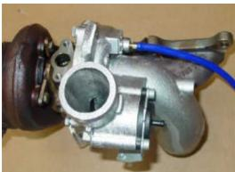
Identify the hose that connects to the turbo compressor housing
