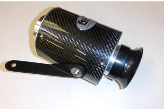
18. You can now fit the carbon air filter and bracket to the vehicle. (The recommended torque setting is between 2 and 2.4NM please do NOT exceed this or the alloy spinning on the filter will deform).
