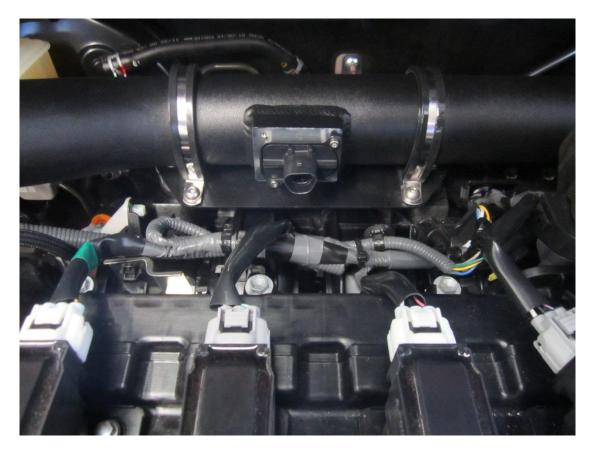
11. Now you can plug the MAF sensor loom back into place and cable tie down the excess loom with the injector loom as shown in the picture below.
