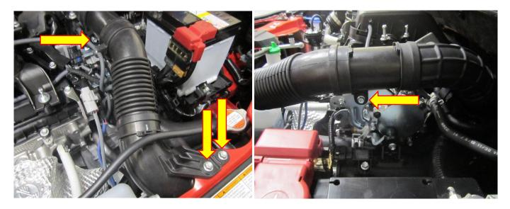
3. Locate the two 10mm fasteners attaching the air box to the engine, remove these with the use of a 10mm spanner. Now remove the vac hose from the air box, this just pulls off.
