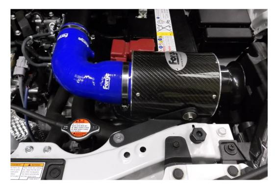
**19**. Finally go back to the mounting bracket and tighten the M6 fasteners and all the hose clamps for the silicone hoses.
