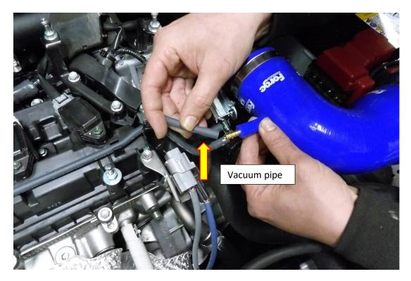
**16**. Remove the 10mm fastener shown in the picture ready to mount the Forge carbon air box.
