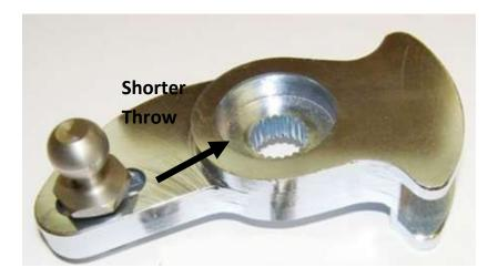
11. Using the grease provided, grease the spine and groove in the shifter.
