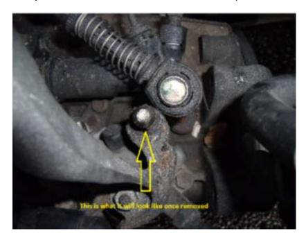
5. Now remove the circular clip on the side next to the gear selector mechanism. This is done by pulling the centre of the clip away and sliding it off at the same time in the same direction.
