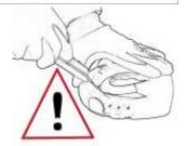
**WARNING** The weld seam must run without gaps along the entire edge of the sole protector to ensure stability.
