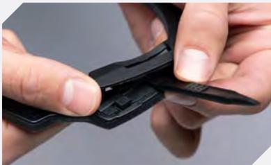
To remove a filter-guide block, use the removal tool that is supplied with the holder system. The pointed end of the removal tool is used to take off the guide-block cover. Once this has been removed, turn the tool round and insert the flat end into the gap in the filter-guide block. This releases the block, which then comes away from the holder with ease.
