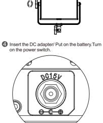
Loosen the U bracket adjusting knob, adjust the angle of the panel which you need, then tighten the U bracket
