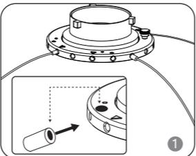
Red dot match: Insert bracket to speed ring adapter, symmetrically install all brackets.
