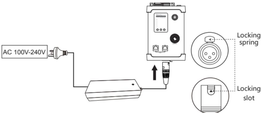
*\* Please pull the power adapter out by pushing the locking spring down on the controller box.*
