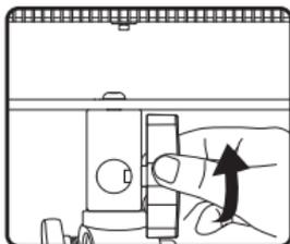
2) Set the light at a specific angle, and pull or turn around the tilt knob to fasten the light.
