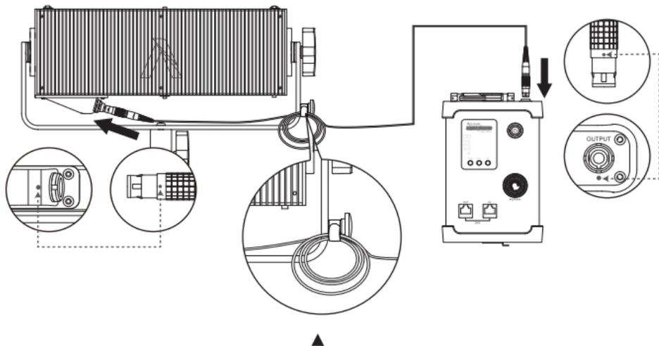
*\*Tie the connect cable around the hook*
