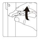
2) Set the light at a specific angle, use clamp handle to fasten the light.
