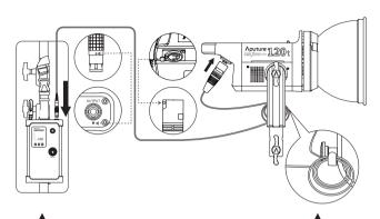
\* Hang the controller box on the tripod by buckle. \* Tie the connecting cable around the hanging column
