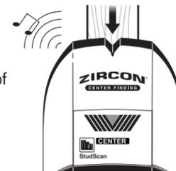
In cases of deeper studs (thicker walls), when the center of the stud is located only two bars will show on the Signal Strength Indicator and only the SpotLite® beam, CENTER indication, and some segments of the Target Indication bars will illuminate. If you still can't locate a stud, try the next step.
