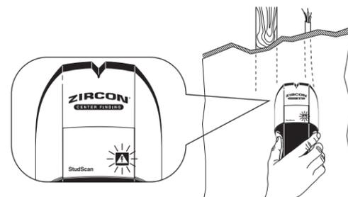
**WARNING** Electrical field locators may not detect live AC wires if wires are more than 2 in. (51 mm) from the scanned surface, in concrete, encased in conduit, present behind a plywood shear wall or metallic wall covering, or if moisture is present in the environment or scanned surface.
