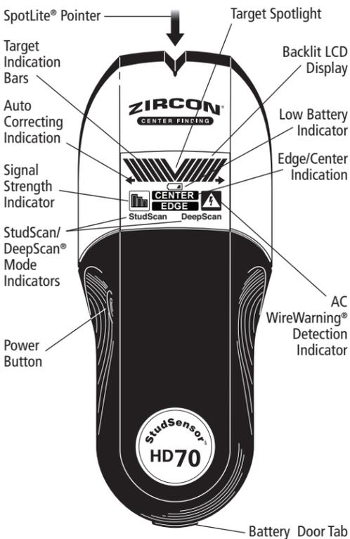
The Zircon StudSensor™ HD70 OneStep® detects both the center and edges of wood and metal studs and joists in walls, floors, and ceilings in one step. It features a blue backlit display, Target Spotlight, and patented SpotLite® Pointer. WireWarning® detection also automatically detects and alerts you of live AC wires.
