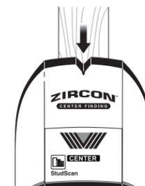
*Note: The tool may detect other objects behind the wall such as pipes and conduit. See Section 2: Operating Tips for ways to confirm that you found a stud.*
