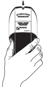
**WARNING** Do not rely exclusively on the detector to locate items behind the scanned surface. Use other information sources to help locate items before penetrating the surface. Such additional sources include construction plans, visible points of entry of pipes and wiring into walls, such as in a basement, and in standard 16 and 24 in. (41 and 61 cm) stud spacing practices.
