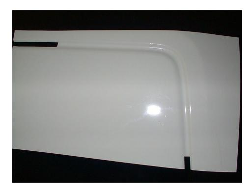
• Illustration of a completed recess corner. Some material has been removed from the recess for clarity.
