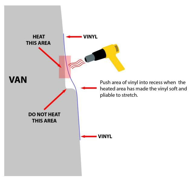
To apply vinyl to a recess, the material should be applied on top of the recess without stretching. The material should then be heated above the recess and the material stretched on the flat/straight section. The material should then be fed into the recess without any need to stretch/stress this area. After application the section should be post heated to "set" the vinyl.
